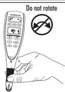
Try to keep the unit in the same upright position while you roll. Rotating the unit while rolling will add or subtract distance.
